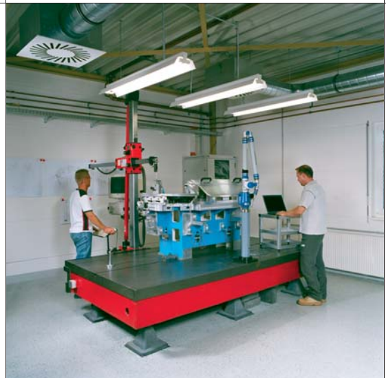
3-D-Measuring technology in the air-conditioned room
